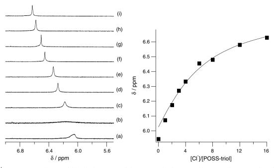
Fig. 4. Partial <sup>1</sup>H NMR spectra of POSS-triol in the absence (a) and the presence of 1 (b), 2 (c), 3 (d), 4 (e), 6 (f), 8 (g), 12 (h) and 16 (i) equiv. of tetrabutylammonium chloride in CDCl<sub>3</sub> at 298 K. [POSS-triol] =  $5.0 \times 10^{-3}$  mol dm<sup>-3</sup>.
