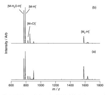
Fig. 5. ESI-MS (negative ion mode) of POSS-triol in the absence (a) and presence of tetramethylammonium chloride (b) in MeCN.
