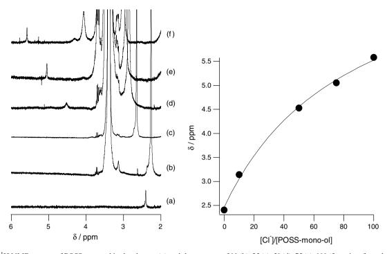
Fig. 8. Partial <sup>1</sup>H NMR spectra of POSS-mono-ol in the absence (a) and the presence of 10 (b), 25 (c), 50 (d), 75 (e), 100 (f) equiv. of tetrabutylammonium chloride in CDCl<sub>3</sub> at 298 K. [POSS-mono-ol] =  $5.0 \times 10^{-3}$  mol dm<sup>-3</sup>.
