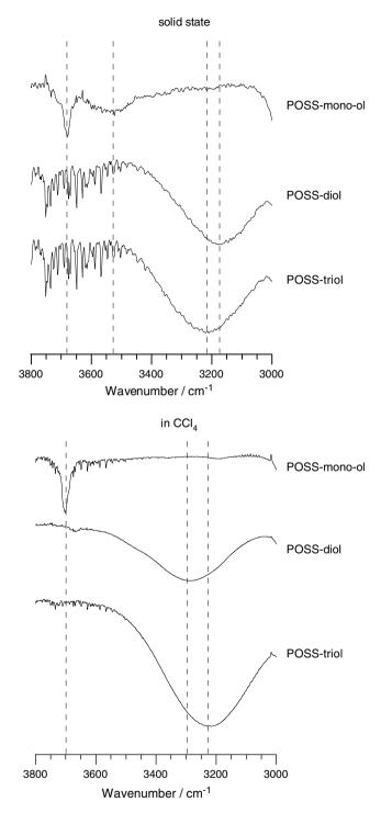
Fig. 3. FTIR spectra of POSS-triol, POSS-diol and POSS-mono-ol in solid state and solution (CCl<sub>4</sub>, 0.1 M).
