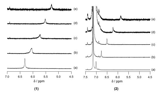
Fig. 1. <sup>1</sup>H NMR dilution experiment in CDCl<sub>3</sub> (1) and in C<sub>6</sub>D<sub>6</sub> (2). [POSS-triol] =  $1.0 \times 10^{-2}$  (a),  $5.0 \times 10^{-3}$  (b),  $2.5 \times 10^{-3}$  (c),  $1.25 \times 10^{-3}$  (d),  $6.25 \times 10^{-4}$  (e) mol dm<sup>-3</sup>.
