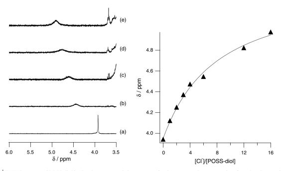
Fig. 6. Partial <sup>1</sup>H NMR spectra of POSS-diol in the absence (a) and the presence of 4 (b), 6 (c), 12 (d), 16 (e) equiv. of tetrabutylammonium chloride in CDCl<sub>3</sub> at 298 K. [POSS-diol] =  $5.0 \times 10^{-3}$  mol dm<sup>-3</sup>.
