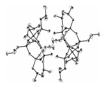
Fig. 9. ORTEP drawing (50% probability) of hydrogen bonded POSStriol dimer. Hydrogen atoms are omitted for clarity.
